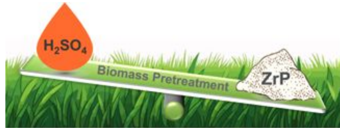
Figure caption: Illustration of the shift from conventional mineral acid pretreatment to a greener, aqueous approach based on solid acid catalysts. Using the image of a balance scale, it emphasizes the substitution of corrosive liquid sulfuric acid with reusable zirconium phosphate in the pretreatment of lignocellulosic biomass. The graphic conveys that heterogeneous solid acids can achieve hydrolysis performance comparable to traditional methods while also allowing easy catalyst recovery and producing sugars that are highly compatible with downstream biological processes.
