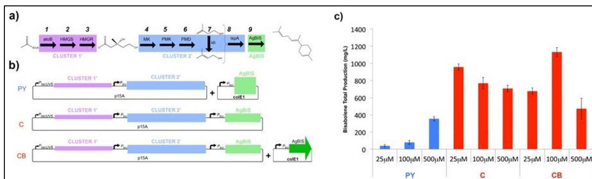
Figure 5. Bisabolene yield improvement (a) pathway description (b) PY, C, CB strains plasmid schematics (c) bisabolene yield from three strains at various IPTG concentrations. From (Alonso-Gutierrez et al., 2015)
