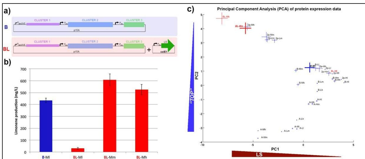
Figure 7. PCAP for limonene yield improvement (a) B and BL strain plasmid schematics (b) limonene yields of B (blue) and BL (red) strains (c) PCA plot with proteomic data and production titer (large cross means high production). B (blue) strain was engineered to improve yield toward BL (red) strain. From (Alonso-Gutierrez et al., 2015)
