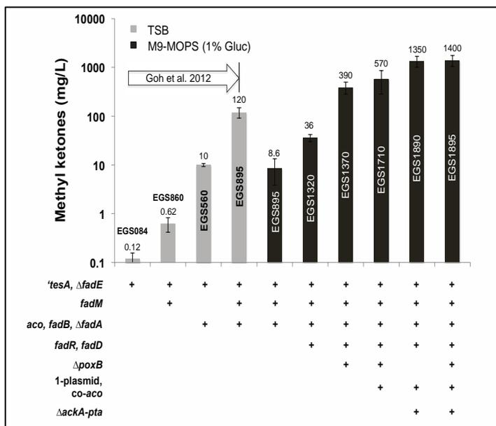
In our best strain to date, a titer of 1.4 g/L of C<sub>11</sub> to C<sub>17</sub> methyl ketones was produced in minimal growth medium with 1% glucose, representing 40% of maximum theoretical yield (Goh et al., 2014). Fed-batch incubations with glucose resulted in ~4.8 g/L methyl ketones (Goh, Beller, *et al.*, unpublished data). These titer and yield values are among the highest reported for any fatty acid-derived fuels or bioproducts.
